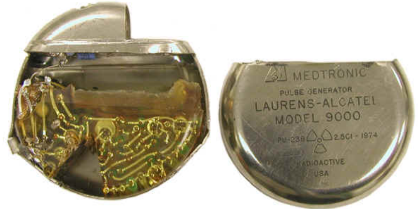
Medtronic plutonium-powered Pacemaker, 1974 (Pu removed)
